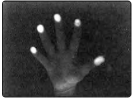
Figure 43: Using FTIR, touch points appear bright to an infrared sensitive camera. Image courtesy of the Natural User Interface Group wiki.nuigroup.com/FTIR
