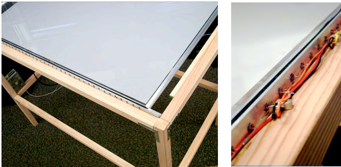
Figure 3: Table construction. Left shows table frame with acrylic sheet and right shows aluminum L channel with LEDs inserted in 5mm holes drilled along edge
